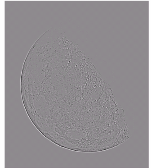
Laplacian Filtered Image Scaled for Display
